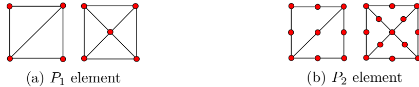
Figure 3.12: A fragment of mesh composed of P_1 and P_2 elements respectively with choice right and crossed diagonal.
