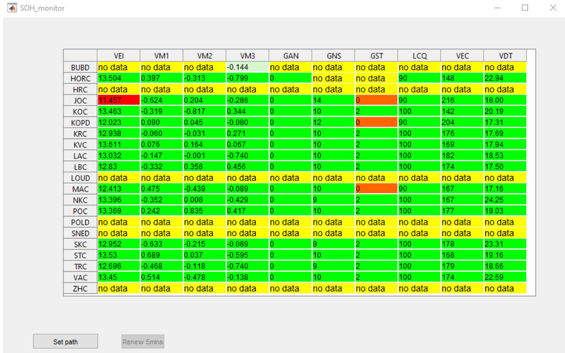
Figure 4.2: SOH Monitor main window. If the values are out of defined limits, the color is changed from green to orange or red (depending on how severe such deviation is). If the SOH data file is not refreshed, the color fades out. If there is no SOH file for current day, the field becomes yellow with 'no data' note.
