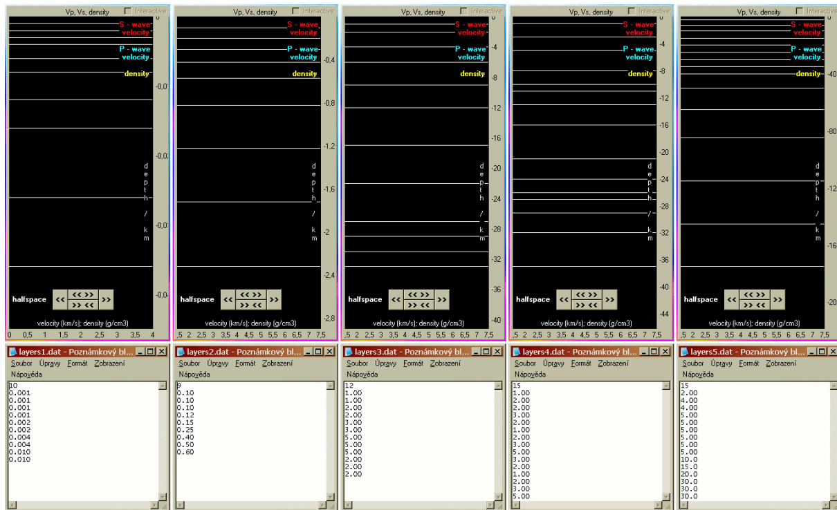
Figure 6.43: Five examples of layer distributions with corresponding input files.
