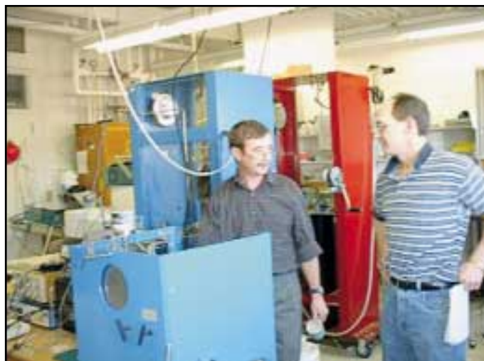
Figure 5. Rock physics laboratory showing pressure vessels used to subject rock samples to in situ pressure conditions. Len Tober (left) and Dean Rokosh (right) are discussing issues related to fluid property measurements.
