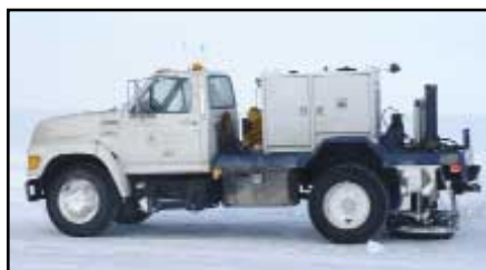
Figure 4. U of Alberta IVI Mini vibrator in action at 69.8°N for the Mallik Gas Hydrate studies in February 2002. Vibrator unit provides 6000-lb peak force with sweep capability from 10-Hz to 500-Hz. The mass can also be mounted horizontally for shear wave generation.
